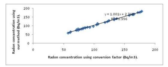
Figure 2: Correlation between the Radon Gas Measurements by the Two Method
